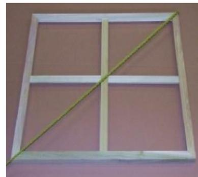
With the frame in front of you hook the end of the tape measure over the back left corner of the frame and measure to the front right corner. Make a note of the length and repeat the process from the back right to the front left corner. Mark the difference between the two distances and hook the tape measure over the two corners with the longest distance between them, adjust the distance by gently tapping with the mallet then check both distances again to make sure your frame is properly square.
