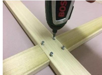
Make sure your fixings are on the side of the cross bars with the rebated ends, so they are not visible from the back of the canvas when the frame is assembled.
